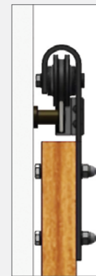
NO HEADER (edge view)
